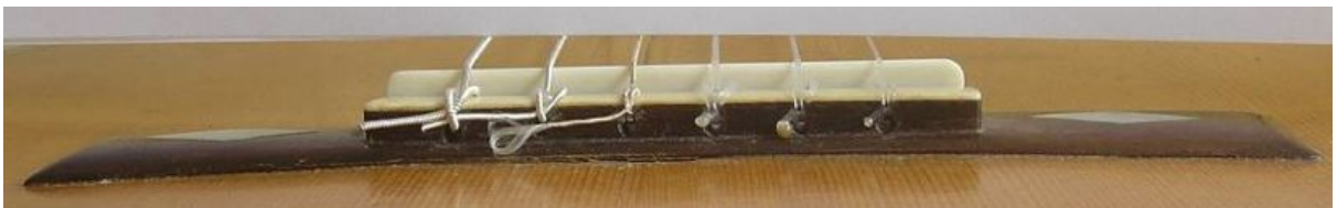
Figure A 25. Doming of the bridge (photo courtesy James Westbrook)
